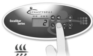
Press and hold **Filter** key until the display shows "xx", representing the currently set filter cycle duration in hours.
