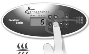
When the desired setting is displayed, press **Filter** key to confirm. A filter cycle starts immediately.
