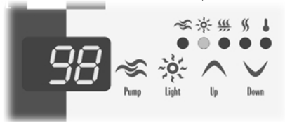
"Heater" & "Set Point" indicator lights
